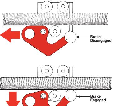
The Fall Protection Block is unpinned and opens up to be put on and taken off of the conductor. The side is secured with a welded hinge pin and push-button locking pin. UHMW rollers, side guides and brake pad prevent the block from causing damage to the conductor.
