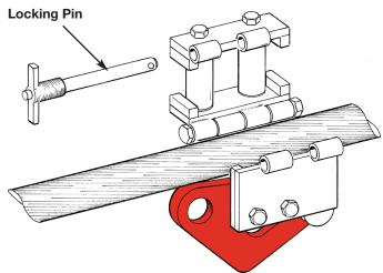
The Lineman's shock absorbing fall protection lanyard is hooked to the ring on the front of the block. The block is pulled down the conductor by the lanyard. In the event the Lineman falls, the shock-absorbing lanyard pulls down on the ring on the front of the block and the brake is applied to prevent the block from running on the wire.
